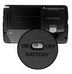
Gently pull the bottom of the GPS receiver away from the iCN.The receiver will lift out to a horizontal position to allow it to obtain a GPS fix.
